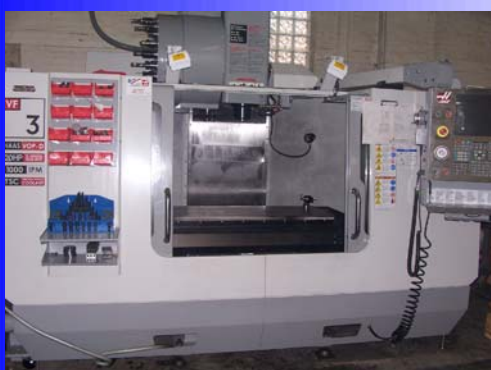
VF-3 vertical machining center has 40" x 20" x 25" xyz travels
